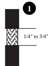
2. Attach Grounding Lead as shown and crimp clip using crimper
