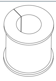
Hanger Grommet with one 28 mm round hole. Suitable for 1-5/8" Hangers and 1-5/8" Double Clamps.
