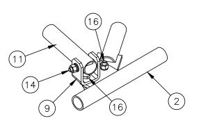
TIE BACK DETAIL AT ANTENNA MOUNTING FRAME
