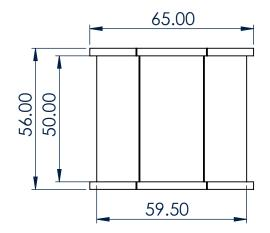
Hanger Grommet with one 8 mm round hole and 7x 12.5 mm holes. Suitable for 2-1/4" Hangers and 2-1/4" Double Clamps.
