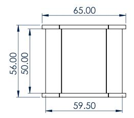
Hanger Grommet with 12x 7 mm round holes. Suitable for 2-1/4" Hangers and 2-1/4" Double Clamps.
