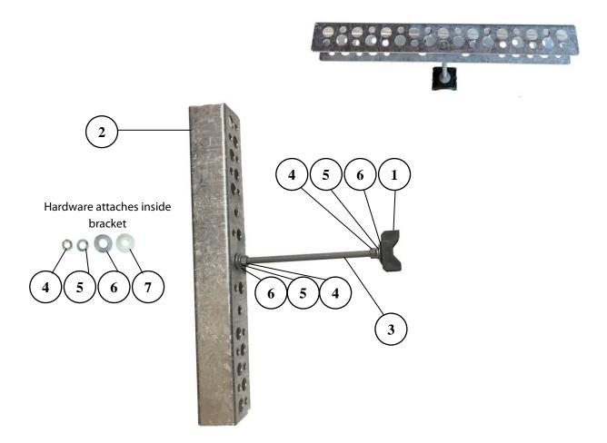
NOTE: For Installations in a high risk PIM zone, approved non-matallic clamps or banding must be used to attach the plastic standoff adapter to the round member.
