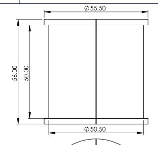
Hanger Grommet with four 12.5 mm and four 7 mm round holes. Suitable for 1-5/8" Hangers and 1-5/8" Double Clamps.
