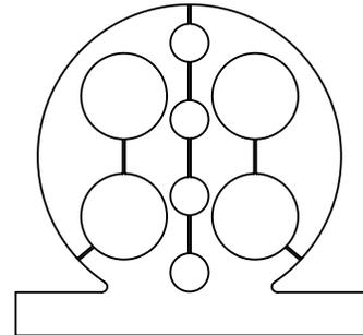
**Round Member Hanger Grommet with four 15.7 mm and four 7 mm round holes.**
