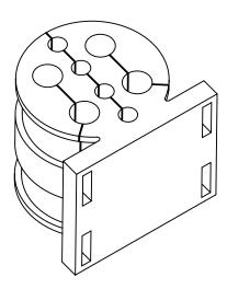
Round Member Hanger Grommet with four 10.9 mm and four 7 mm round holes.
