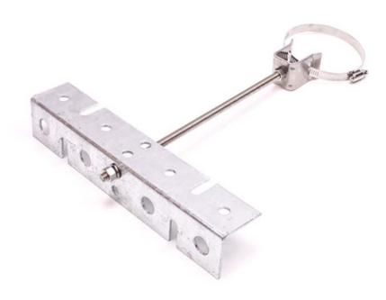
Tower Stand Off, 3/8" Threaded Hole Hose Clamp for 2-3/8" to 4" OD Round Member 12" Trapeze Angle 3/8" x 12" Stainless Steel Threaded Rod 3/8" Stainless Steel Nuts 3/8" Stainless Steel Lock Washer
