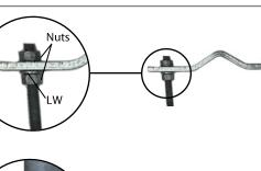
Low PIM Cable Support Bracket Kit shown with Double Clamps and
