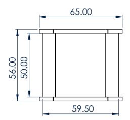
Hanger Grommet with one 8 mm round hole and 9x 10.9 mm holes. Suitable for 2-1/4" Hangers and 2-1/4" Double Clamps.
